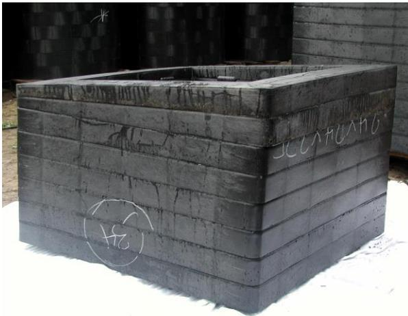
3. Combine various ring heights, in both flat and slope, to reach desired adjustment. Rings are to be placed with pocket openings down and tabs extending into structure or lower rings. Note: Slope rings are tapered from side to side at an angle to provide a 1% to 3% grade compensation.
